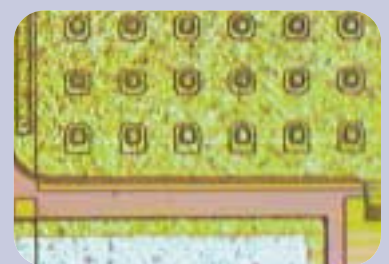
Optical micrographs of part of an automobile engine management control pcb (Field of view 2cm and 200 \mu\text{m} )
